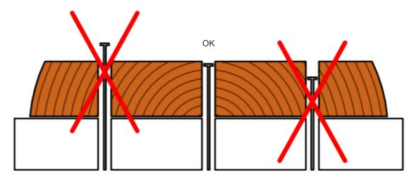
Recommended head penetration when fixing ThermoWood cladding.
