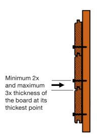
Minimum 2x and maximum 3x thickness of the board at its thickest point
