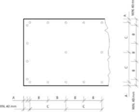
Required distances as a function of the most frequently used board thicknesses
