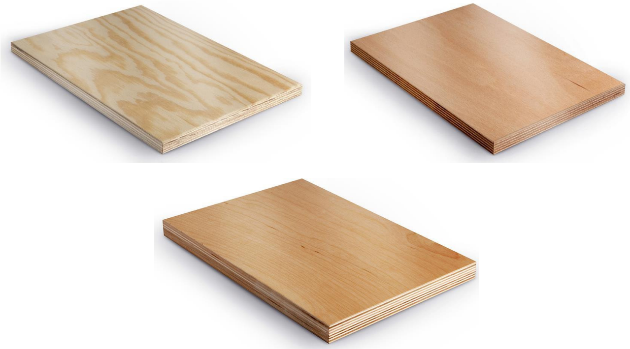
Fig. 2. A pine plywood sheet (top, left side), beech plywood sheet (top, right side) and birch plywood sheet (bottom) produced by Sklejka – Multi.
